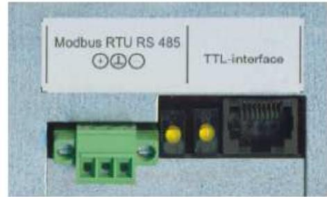
The power supply of the Modbus extension has the same voltage range as the main device. Due to this the supply voltage can be taken from the voltage terminals. Please consider the labels on the device.
