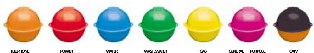
Engineered for narrow trench applications up to five feet in depth, the four-inch diameter ball marker has a unique, patented self-leveling feature that ensures an accurate, horizontal position regardless of how it is placed in the ground. (Contains a mixture of Propylene Glycol and water which is approved for use in pharmaceuticals, cosmetics and as a food additive. The mixture is readily biodegradable and will not harm humans, wildlife or the environment.)
