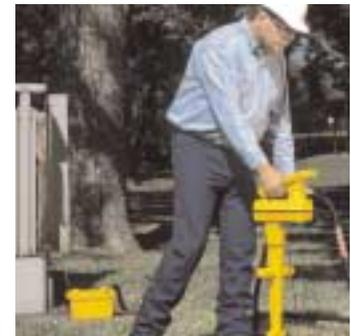
**Tailored to Meet Your Needs.** The new 3M Dynatel 2200M Series Locators offer several features for cable/pipe locating with more accuracy, speed and sensitivity than ever. These receivers provide two directional modes: Directional Peak and Directional Null; plus an ultra-sensitive Single Peak mode for extreme depths. They also incorporate an “expander” function to make peaks and nulls more pronounced by enhancing the amplitude difference between two conductors carrying the same tone.
